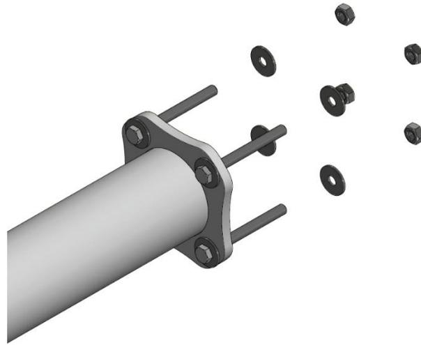
**8.** On each of the four M10x100 hexagon screw (10), slide on washer M10 (9) and insert the hexagon screw M10x100 (10) through the holes of the flange.
