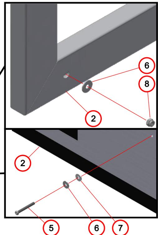
3. Tighten the backboard (2) to the posts (1) with four countersunk screws M8x80 (5), eight washers M8 (6), four polyamide discs M8 (7) and four hexagonal nuts M8 (8)
